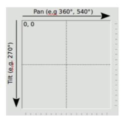
There are cases though where you want to limit the degrees a moving head or a scanner could reach. For example fixtures with a 540° Pan range, should be limited to work only in a range facing the audience, or you might want to avoid that moving heads mounted upside down on a truss will point to the ceiling or outside the stage.
