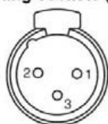
DMX - output XLR mounting-sockets (rear view):
